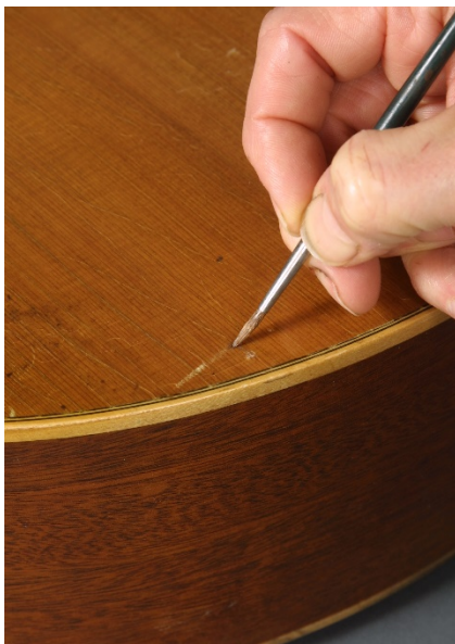
A big feature of lacquer is repairability. Here, thinned lacquer is applied to a lacquer finish to repair a scratch.
