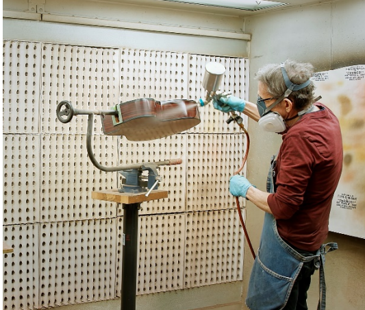
The author applying clear finish in a spray booth. Photo by Angelo Merendino Photography.
